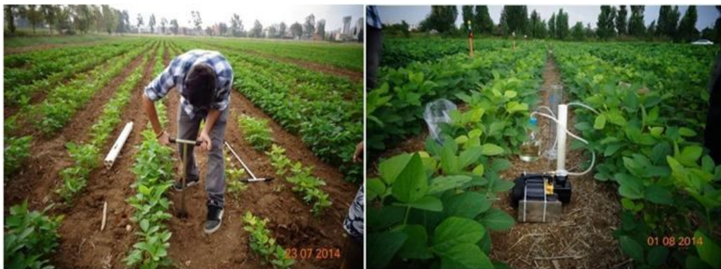
Figure 2. Placing a soil water sampler on a research plot. Water was collected after each of the irrigation and rain event.
