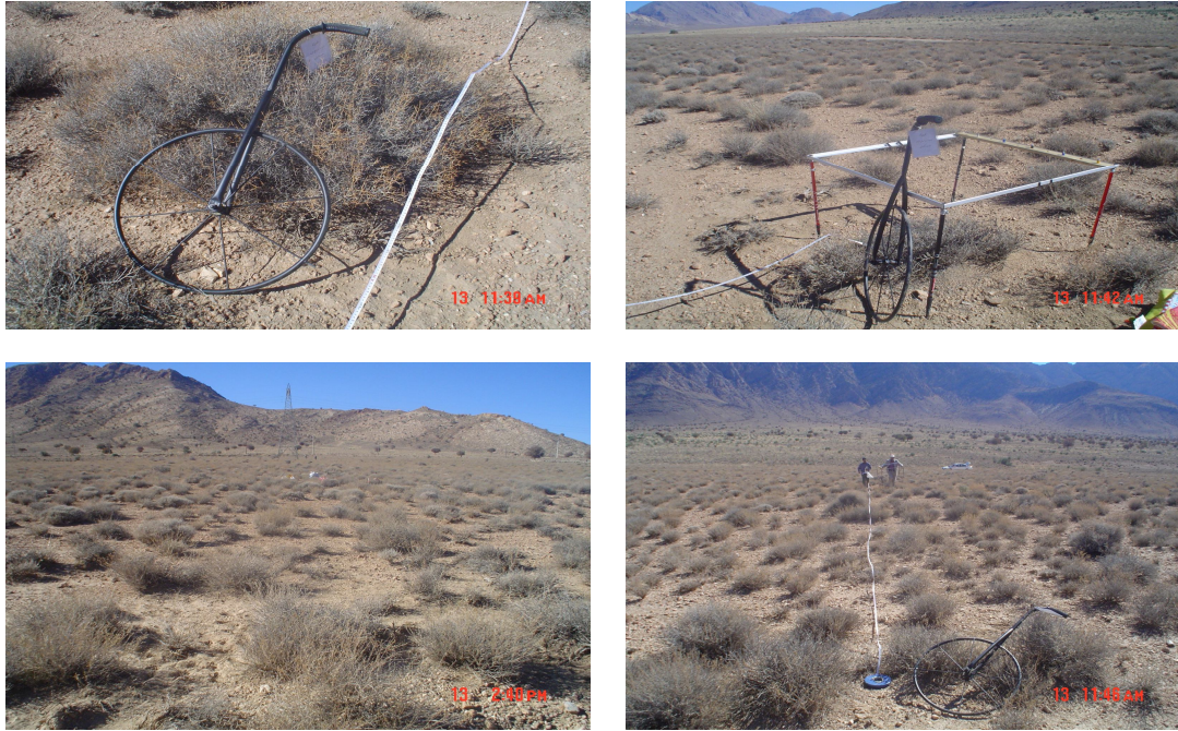
Figure 2. Images of wheel-point device designed for sampling and the Artemisia sieberi stands studied.
