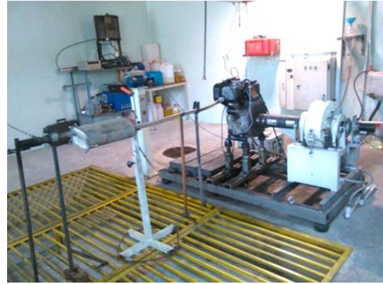
Figure 3. Performing engine performance tests with a dynamometer
