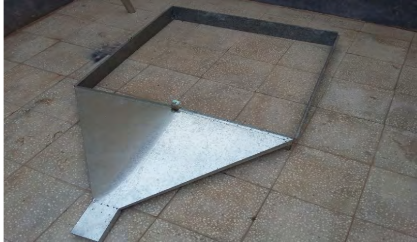
Figure 2. The erosion plot consists of 1m×1m galvanized plates
